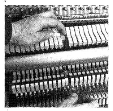
Figure 2: Since bass hammers do not match the angle of their strings, they cross the strings slightly. If each hammer is not centered exactly to its unison, it may contact a neighboring unison string. The easiest way to judge bass hammer alignment is just to look at the gap between the top right corner of each hammer and the next string to the right, and the lower left corner and the next lowest string, and
